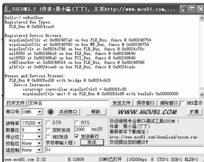
Figure 8 Diagram of drive device hook up
